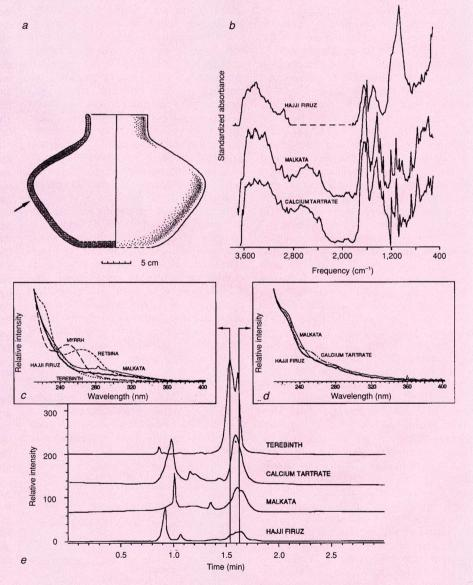
IR spectrum was obtained by a micro technique. The liquid chromatograph was run at ambient temperature, using a  $25 \text{ cm} \times 4.6 \text{-mm}$  silica column, a flow rate of 2.0 ml per min, and an UV detector over the 200-400 -nm range. Variation in the retention times of earlier peaks (0.9-1.1 min) on some chromatograms (e) is probably due to the different temperatures of individual analyses, as well as interactions in complex mixtures.
