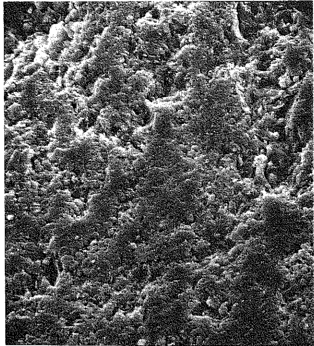
Plate 4 b: SEM image of interior of BC-7 (magn., 800X), after refiring to 700^\circ\text{C} . Note the extensive areas of sintering.
